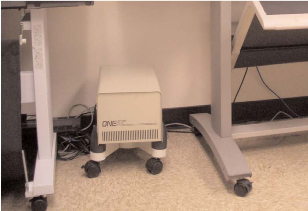
One of ONEAC's UPS's that was placed in Franco's site to help correct the issues with his equipment.
